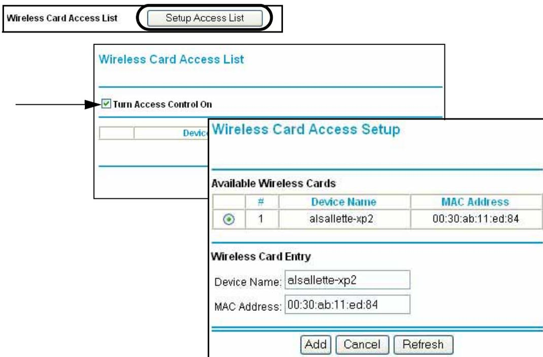
Figure 4-5: Wireless Card Access List Setup
